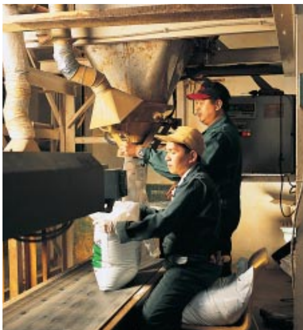
The bag-filling operation at Evergro Products plant often goes through several changeovers per day to accommodate a wide range of bag sizes shipped from the facility.
