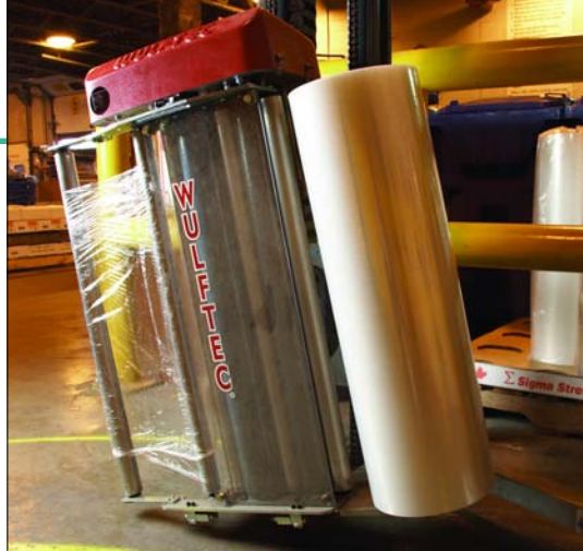
The installation of two WRT series stretchwrapping systems has enabled the Sysco-Vancouver distribution center to reduce its consumption of stretchwrap film by about a third, providing a very quick payback for the new equipment.
