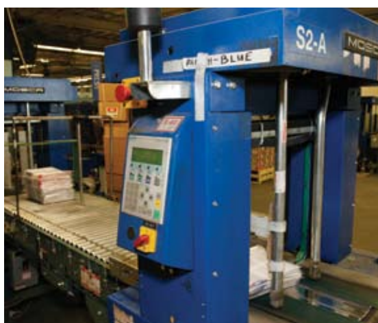
A Siemens Simatic OP7 programmable logic controller ensures optimal control and efficiency on the Mosca strapping machine.
