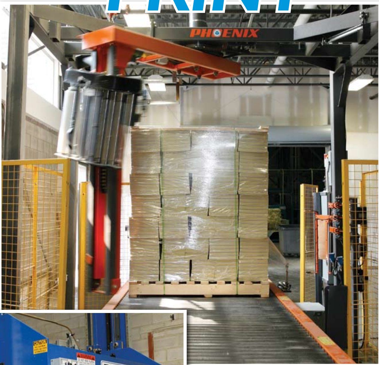
A state-of-the-art PRTA-2200 conveyorized rotary-arm automatic stretchwrapping machine makes quick work of securing a load of catalogs at the end-of-the-line packaging area of the Quebecor World Islington plant in west-end Toronto.
