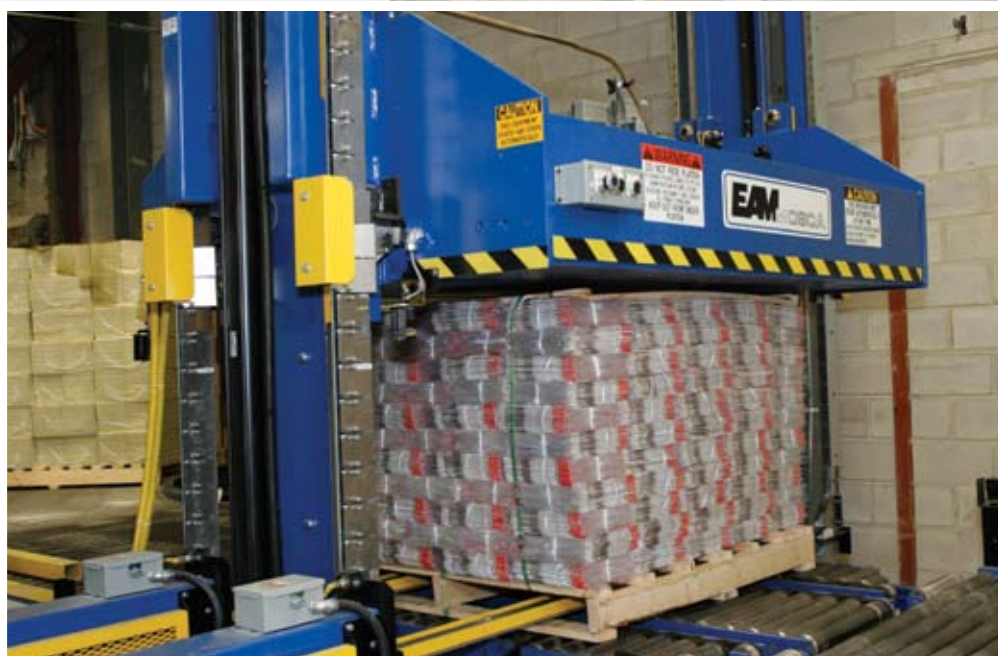
Applying 12,000 pounds of hydraulic compression force to a palletized load of printed materials, the CTS 602-10 strapping machine secures a pair of plastic straps to the load before turning it 90 degrees for cross-strapping.
